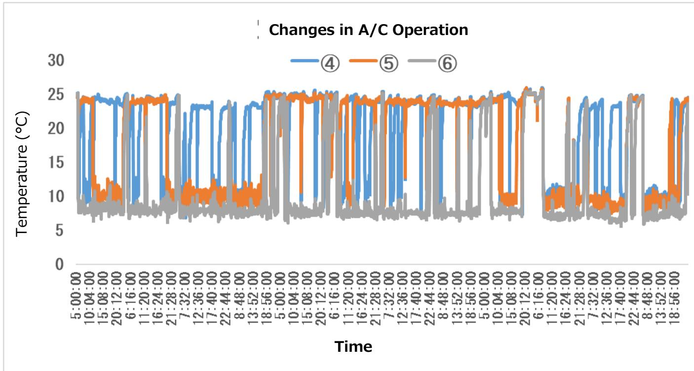
From the figure, it can be seen that the three air conditioners were operating separately. The stop time was longer than without the Air film, and the average temperature was  $18.1^{\circ}\text{C}$ ,  $2.0^{\circ}\text{C}$  higher. The temperature difference from 1 cm from the window was  $7.6^{\circ}\text{C}$ ,  $2.3^{\circ}\text{C}$  smaller than without the Air film.
