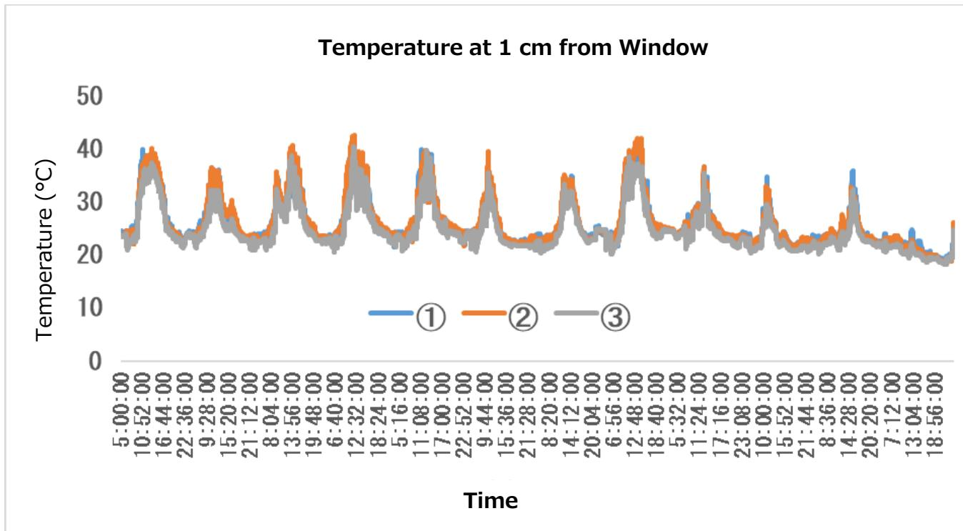
The average temperature at 1 cm from the window was 25.7°C, 0.3°C lower than without the Air film.
