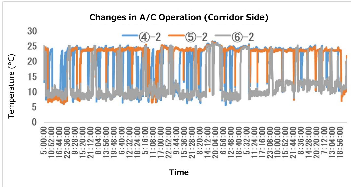
From the figure, it can be seen that the three air conditioners were operating separately. The stop time was longer than without the Air film, and the average temperature was 18.4°C, 2.1°C higher. The difference from the corridor side temperature was 5.1°C, 2.9°C smaller than without the Air film.
