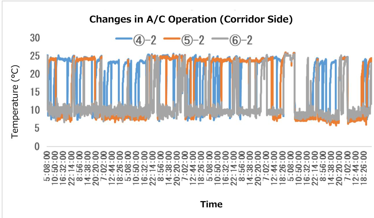
From the figure, it can be seen that the three air conditioners were operating separately. The average temperature was 16.3°C, giving a difference of 7.0°C from the corridor side temperature.
