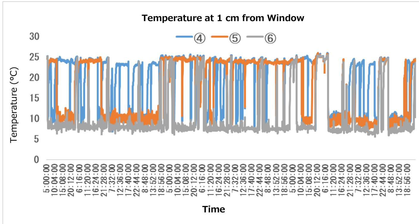
From the figure, it can be seen that the three air conditioners were operating separately. The average outlet temperature was 16.1°C, the temperature at 1 cm from the window was 26.0°C, giving a difference of 9.9°C.
