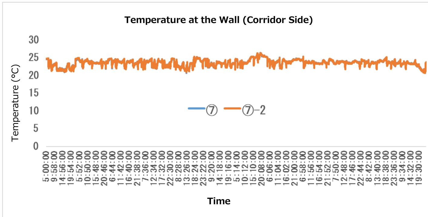
The average temperature was 23.5°C, 0.2°C higher than without the Air film (23.3°C).
