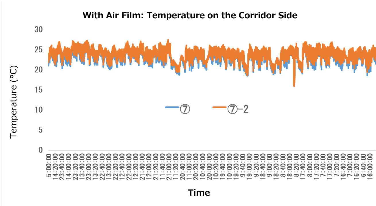
The average temperature was 23.5°C, which was 0.4°C lower than the measurement without the Air film (23.9°C).
