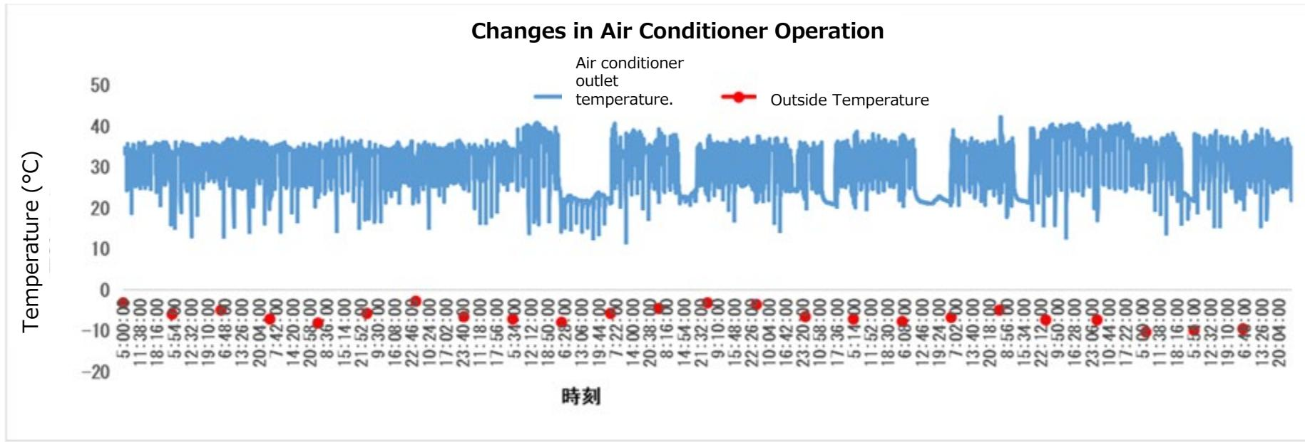
The AC unit stopped operating when the outside temperature rose to -4°C or higher.
