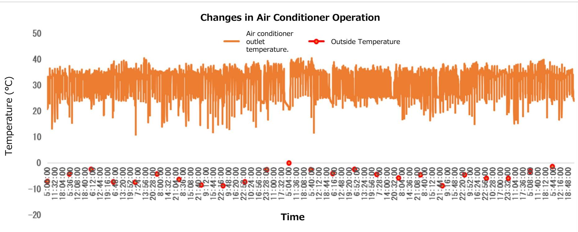
The AC unit stopped operating for approximately 4 hours, but only when the outside temperature was 0°C or higher (0.1°C).
