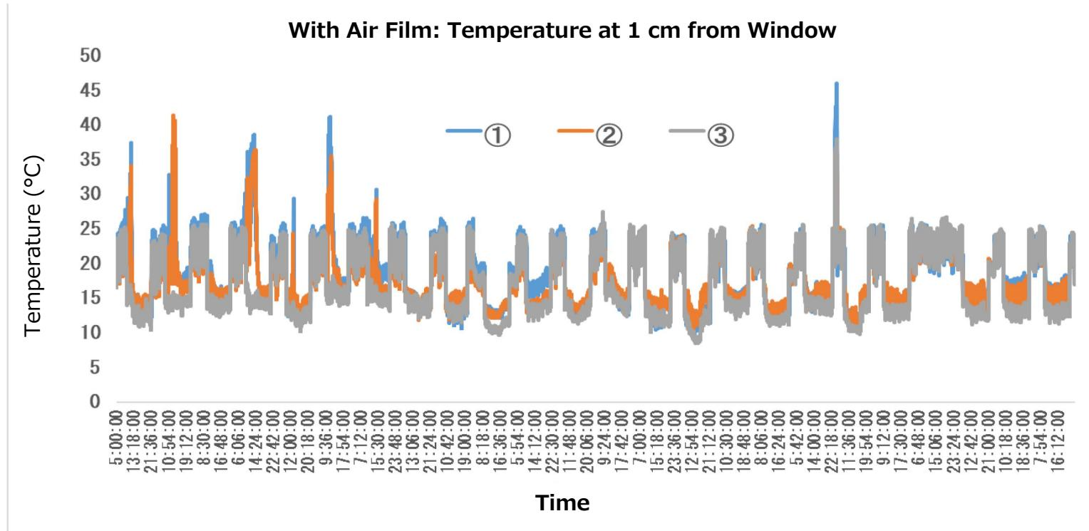
The average temperature 1cm from the window was 17.7°C, which was 0.8°C higher than the measurement without the Air film.
