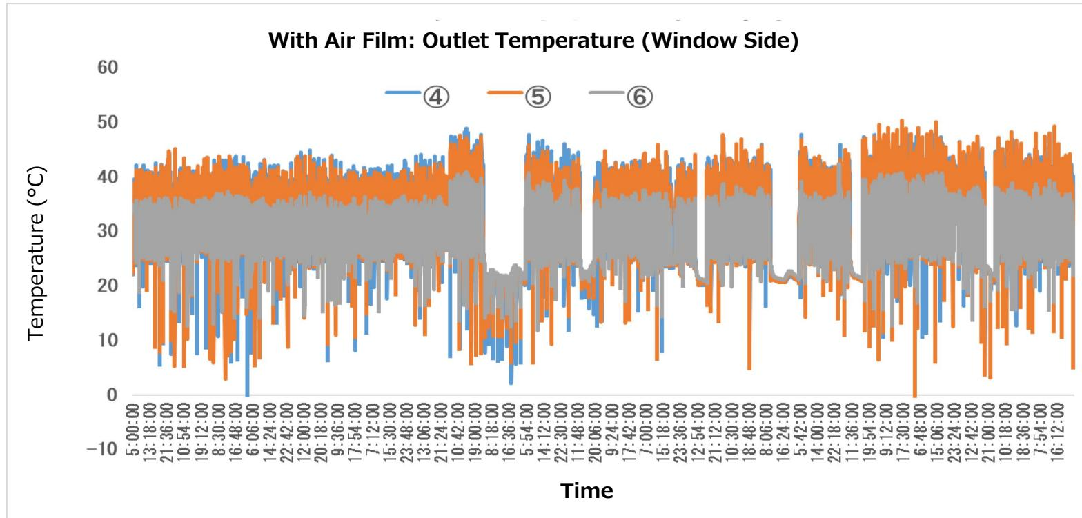
The graph shows that all three AC units were operating simultaneously.
