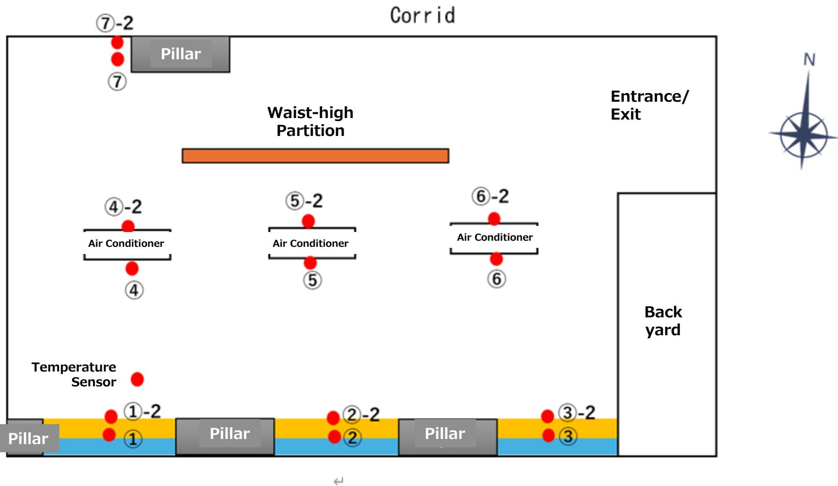
Temperature at 1 cm and 5 cm from the window surface (2 points each): glass side Air conditioner outlet (2 points each)
